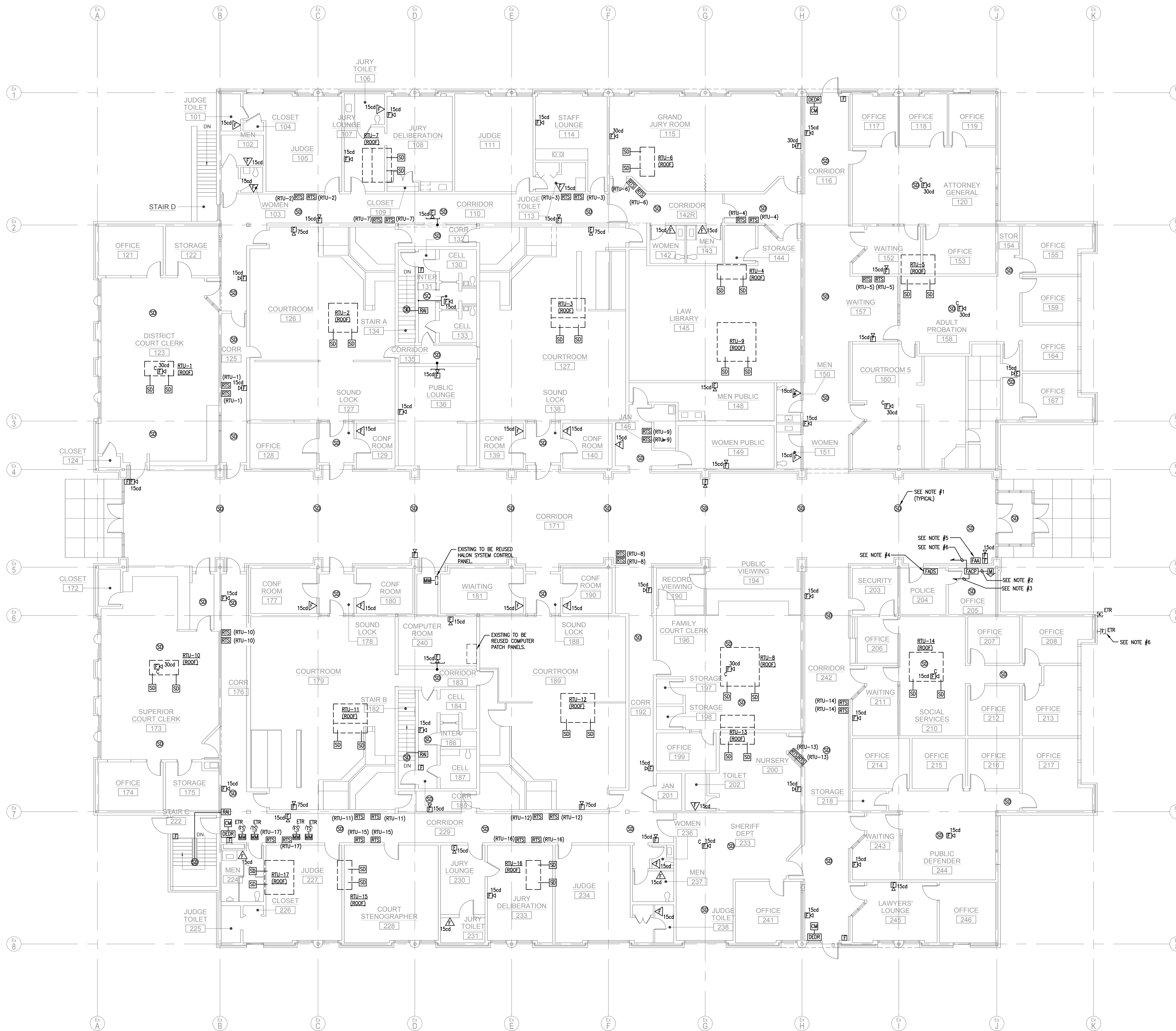
1 FIRST FLOOR FIRE ALARM PLAN E1.01 SCALE: 1/8" = 1'-0"
